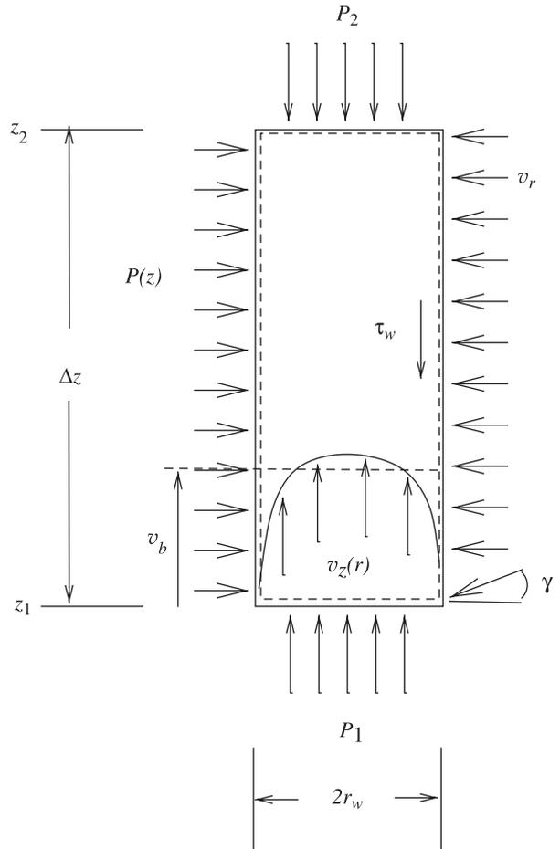
**Figure 7. Momentum balance control volume for a wellbore.**
