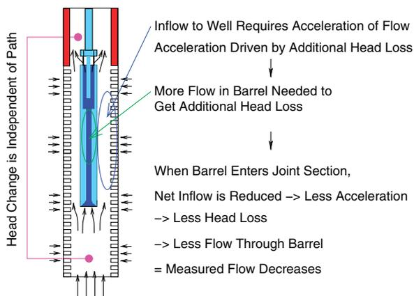
**Figure 10. Diagram of physical phenomena influencing flowmeter measurements when inflow to the borehole occurs.**
