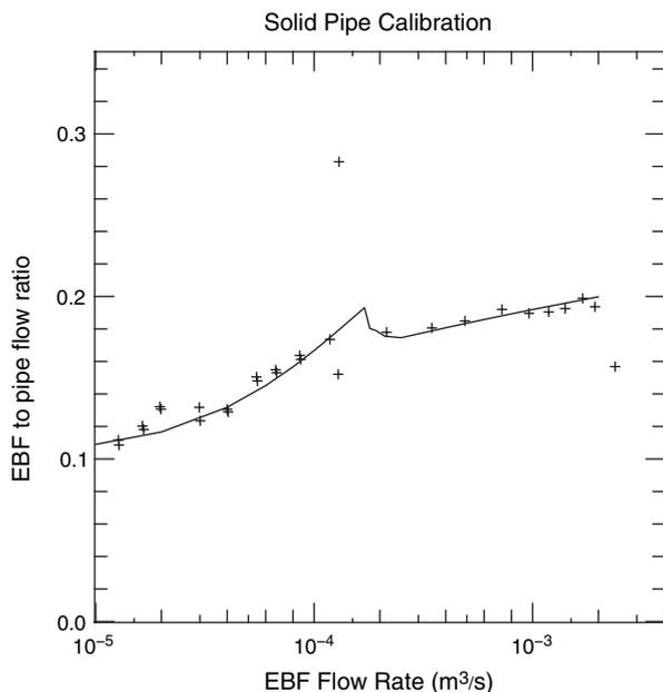
**Figure 3.** Flowmeter measurements from solid pipe calibration (symbols) and calculated flowmeter response (line).
