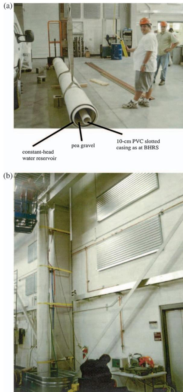
**Figure 4.** (a) Borehole-aquifer simulator and (b) simulator configuration during experiments.
