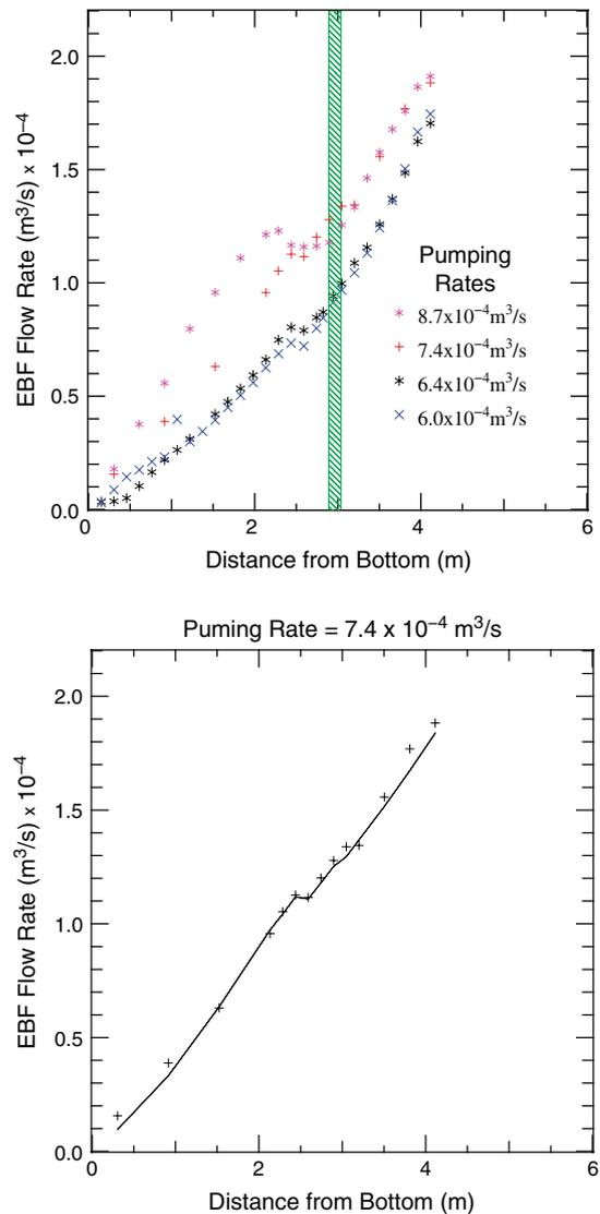
**Figure 5. (a) Selected experimental data sets. The shaded vertical line indicates the position of the casing joint and (b) data (symbols) and calculated flowmeter response (line).**
