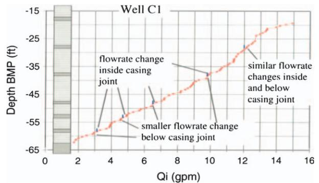
**Figure 2.** Example of anomalous flowmeter measurements.
