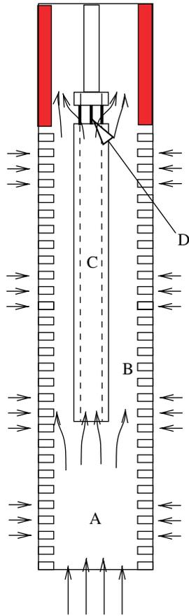
**Figure 6. Regions of different flow conditions: location A, flow in an open borehole; location B, flow around the flowmeter barrel; location C, flow inside the flowmeter barrel; location D, flow exiting the flowmeter barrel.**
