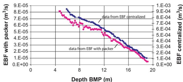
**Figure 1.** Comparison of EBF measurements for the same well using a packer (lower data set; left axis) and with a centralizer (upper data set; right axis). The measurements with a packer are more noisy, probably due to much smaller flow rates. Note that the pumping rate was over an order of magnitude larger when the centralizer data were acquired (right axis). Data shown here are full-recorded flow rates, not net flowrates following removal of ambient flow.
