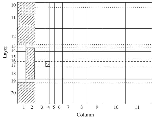
**Figure 9. Example discretization of model. Shaded regions above layer 19 represent no flow regions of the flowmeter or in the case of column 4 a blank section of well screen and below layer 19, columns 1 and 2 are not part of the model and the inner diameter of column 3 set to 0.**
