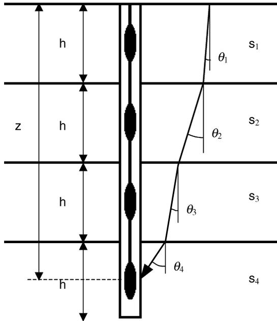
Figure 1. Schematic diagram illustrating the parameters used for the curved-ray forward model. Each layer has a thickness of  $h$  and slowness of  $s_n$ . The angle between the segment of the ray in layer  $n$  and the vertical is  $\theta_n$ . The depth of the receiver is  $z$ .
