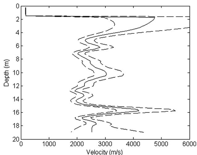
Figure 6. Final velocity model produced by curved-ray inversion of the C4 RVSP data set. The solid line is the velocity model; the dashed lines are the 95% confidence intervals. Above  $\sim 4$  m and below  $\sim 16$  m, the velocities are unrealistic and the uncertainties are great.
