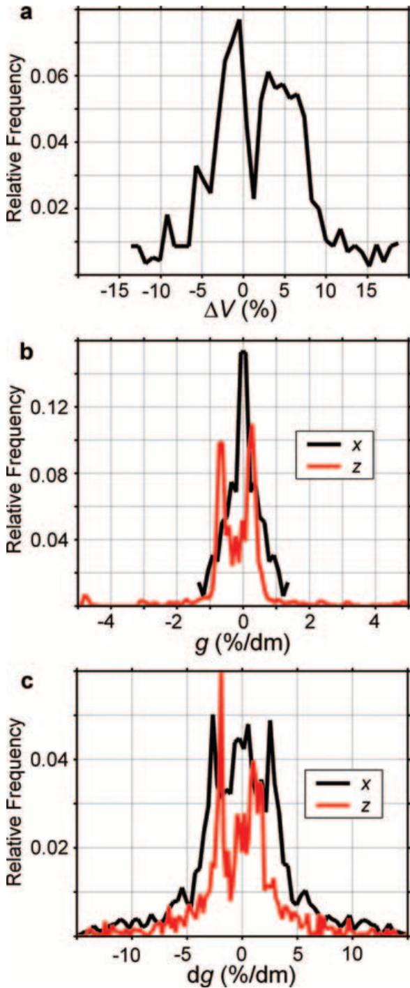
**Figure 8.** Distribution of (a) the relative change in the data from a homogeneous background, (b) the relative sensitivity of the data to receiver position, and (c) the relative sensitivity of the differenced data to receiver position for the pole–pole experiment. The legends *x* and *z* indicate sensitivity in the horizontal and vertical directions, respectively.
