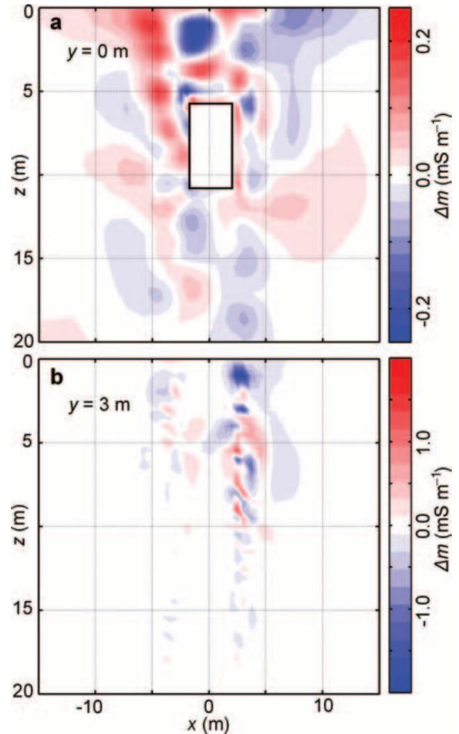
**Figure 11.** Pole-pole conductivity artefact distributions in the planes of (a) the target ( $y = 0$  m) and (b) the mislocated electrode ( $y = 3$  m) for a 0.25 m vertical mislocation of the uppermost electrode of BH1. Location of the conductive target is outlined.
