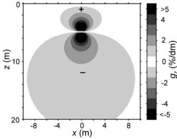
**Figure 1.** Normalized sensitivity of potential to receiver electrode position in the vertical direction for a pole-pole experiment. The current source is located at  $x = 0$  m,  $z = 5$  m within a 3-D half-space. For example, a 10 cm vertical mislocation of a common-hole receiver pole at 10 m depth would result in approximately 2 per cent error in the datum.
