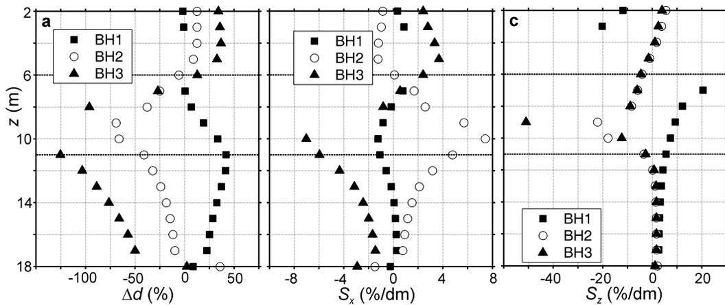
**Figure 6.** Vertical dipole-dipole synthetic experiment with the source dipole centred at 5.5 m depth in BH1. (a) Relative change in data from homogeneous background condition. Relative sensitivity of data to (b) horizontal and (c) vertical receiver dipole position. Quantities are plotted at the uphole electrode.
