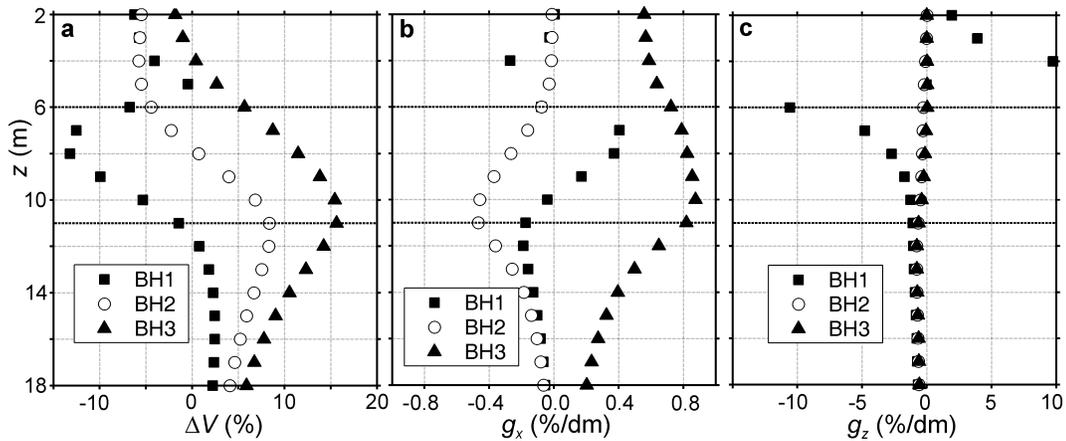
**Figure 5.** Pole-pole synthetic experiment with the source located at 5 m depth in BH1. (a) Relative change in data from homogeneous background condition. Relative sensitivity of data to (b) horizontal and (c) vertical receiver position. Dashed lines indicate vertical limits of heterogeneity.
