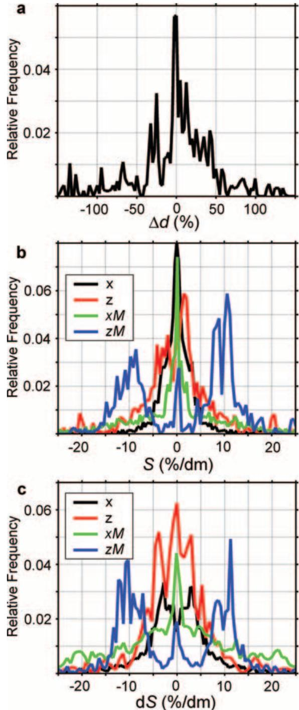
**Figure 9.** Distribution of (a) the relative change in the data from a homogeneous background, (b) the relative sensitivity of the data to position of the receiver dipole and the positive receiver electrode *M* and (c) the relative sensitivity of the differenced data to position of the receiver dipole and the positive receiver electrode for the vertical dipole–dipole experiment. The legends *x* and *z* indicate sensitivity in the horizontal and vertical directions, respectively.
