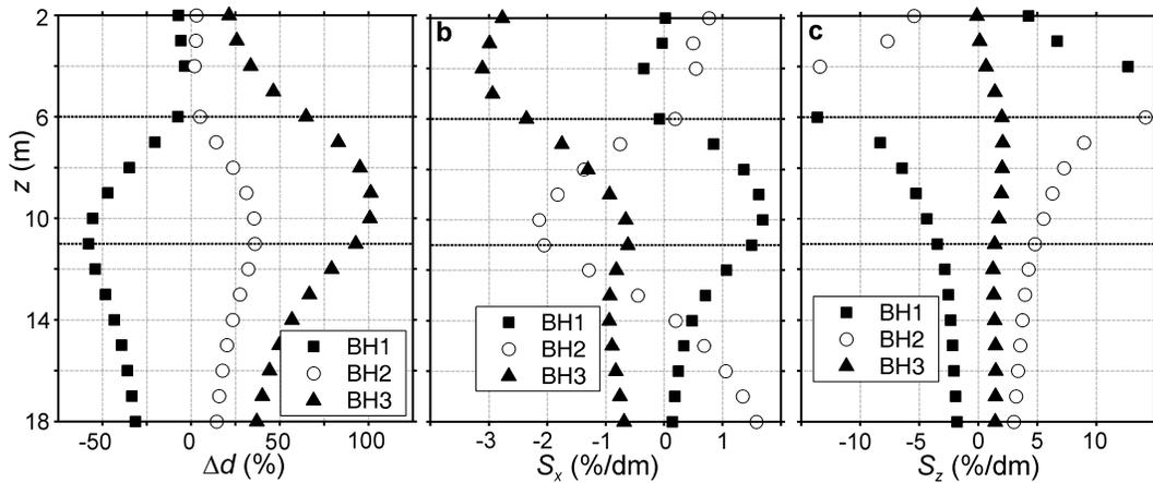
**Figure 7.** Horizontal cross-borehole synthetic experiment with the source dipole at 5 m depth spanning BH1 and BH2. (a) Relative change in data from homogeneous background condition. Relative sensitivity of data to (b) horizontal and (c) vertical receiver dipole position. Quantities are plotted at the positive receiver electrode.
