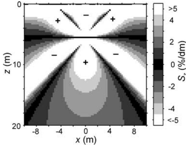
**Figure 2.** Normalized sensitivity of potential difference to vertical position of the receiver dipole for a vertical 1 m dipole-dipole experiment. The current dipole is centred at  $x = 0$  m,  $z = 5.5$  m. Sensitivities are plotted at the receiver dipole centre. For example, a 10 cm vertical mislocation of a common-hole receiver dipole at 10 m depth would result in greater than 5 per cent error in the datum.
