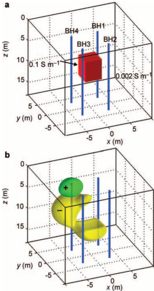
**Figure 4.** (a) Synthetic experimental geometry. (b) Sensitivity of potential to vertical receiver position for a pole-pole experiment. The figure illustrates perturbation of the  $\pm 1$  per cent/dm sensitivity isosurfaces for a source electrode at 5 m depth in BH4.
