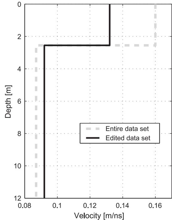
Fig. 9. Inverted two-layer velocity model using the entire traveltimes data set (RMS residual 2.76 ns) compared to one using the data set in which potential critically refracted arrivals are eliminated in analogy to Fig. 8b (edited data set, RMS residual 0.84 ns).
