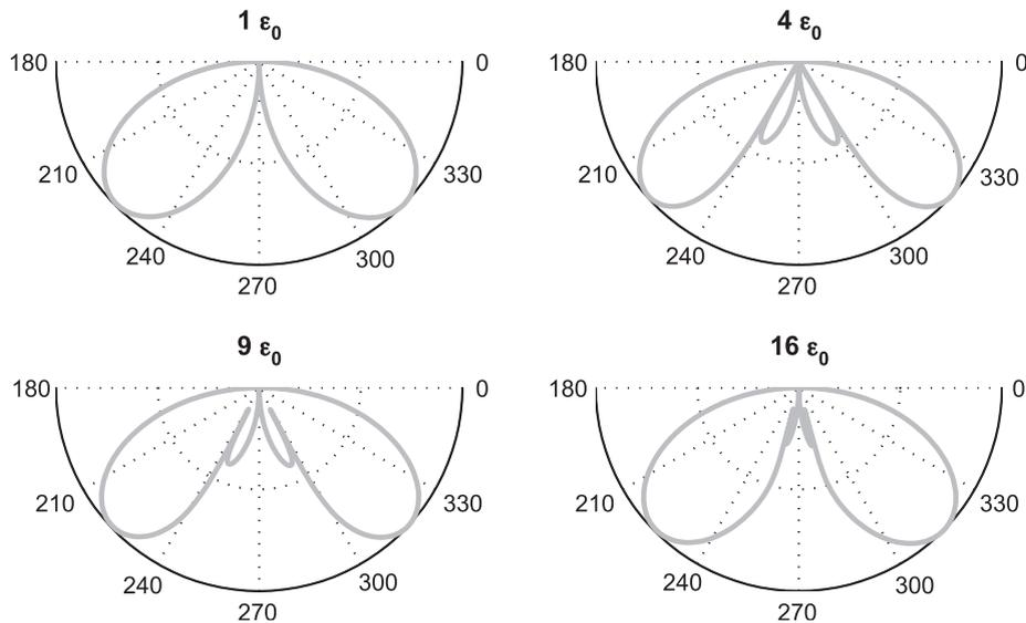
Fig. 6. Influence of subsurface dielectric permittivity on the amplitude sensitivity of the VRP antenna configuration. Radiation patterns are the result of combining the analytical far-field radiation patterns of an infinitesimal horizontal dipole with that of an infinitesimal vertical dipole. Different diagrams represent different subsurface dielectric permittivities (values shown above each plot). Each curve is normalized to its individual maximum value. For angle definition, see Fig. 4.
