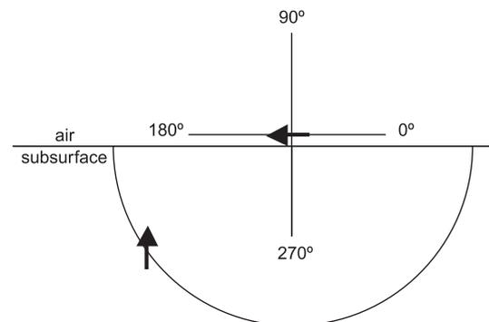
Fig. 4. Sketch illustrating antenna layout in a typical VRP experiment. The horizontal surface dipole antenna is represented by the horizontal arrow and the vertical borehole dipole by the vertical arrow.
