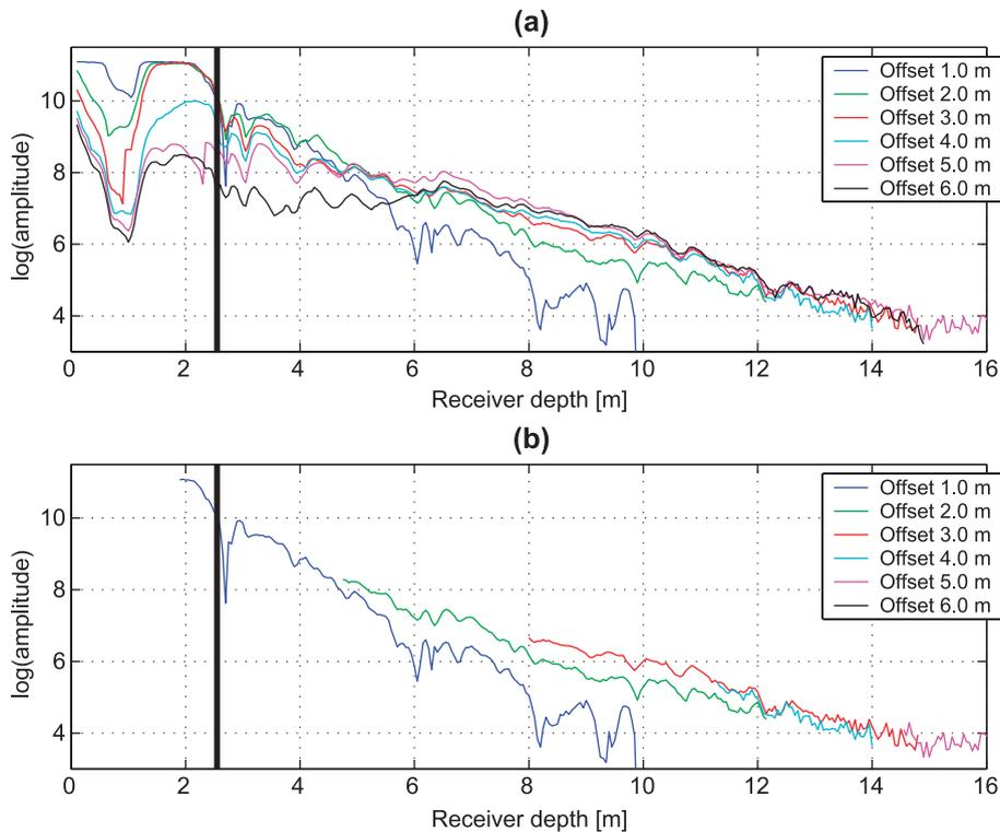
Fig. 8. First cycle amplitudes as a function of receiver depth for all measured transmitter offsets. In (a), all picked data are shown, whereas in (b), data are only plotted for depths where no critically refracted arrivals are expected. The thick solid lines at a depth of 2.55 m represent groundwater table depth. For details, see text.
