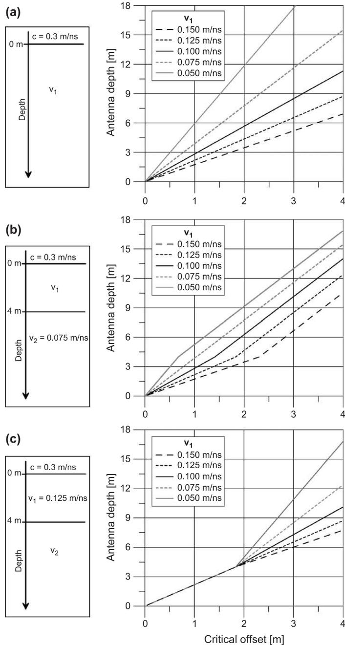
Fig. 2. Critical offset from borehole as a function of receiver-antenna depth for three suites of three-layer models: (a) air and homogeneous layer with thickness  $>18$  m and a homogeneous half-space (latter not shown in model sketch); (b) air, 4.0-m-thick layer with variable velocity and a homogeneous half-space with a 0.075 m/ns constant velocity; (c) air, 4.0-m-thick layer with constant 0.125 m/ns velocity, and a homogeneous half-space with variable velocity.
