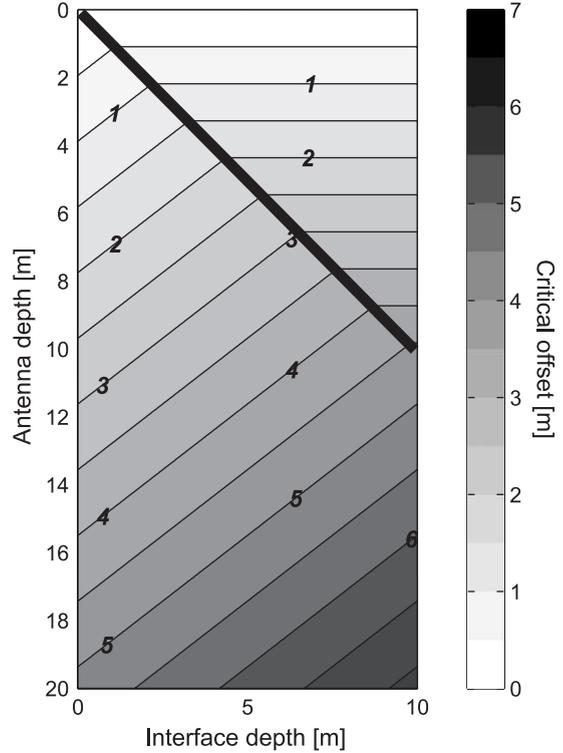
Fig. 3. Critical offset from borehole as a function of receiver-antenna and interface depths for a three layer case:  $c=0.3$  m/ns (air),  $v_1=0.125$  m/ns and  $v_2=0.075$  m/ns. The black line separates antenna positions above the interface from those below.
