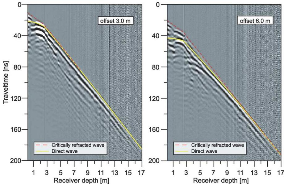
Fig. 7. Two common transmitter gathers of the BHRS data set recorded at different borehole offsets. The two gathers are displayed with the same depth-scaled gain. Overlain curves show arrival times for the critically refracted waves (dashed red curves) and for the direct waves (solid yellow curves) calculated using a simplified model consisting of air ( $c=0.3$  m/ns), a 2.55-m-thick homogenous layer ( $v_1=0.14$  m/ns) and a homogenous half-space ( $v_2=0.09$  m/ns).
