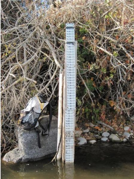
**Figure 4: Downstream river staff gauge and stilling well at low stage, gauge increments are 0.02 ft.**
